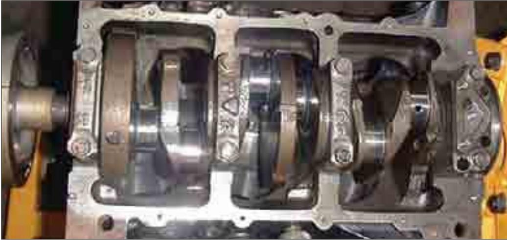
Crankshaft inside the crank-case
