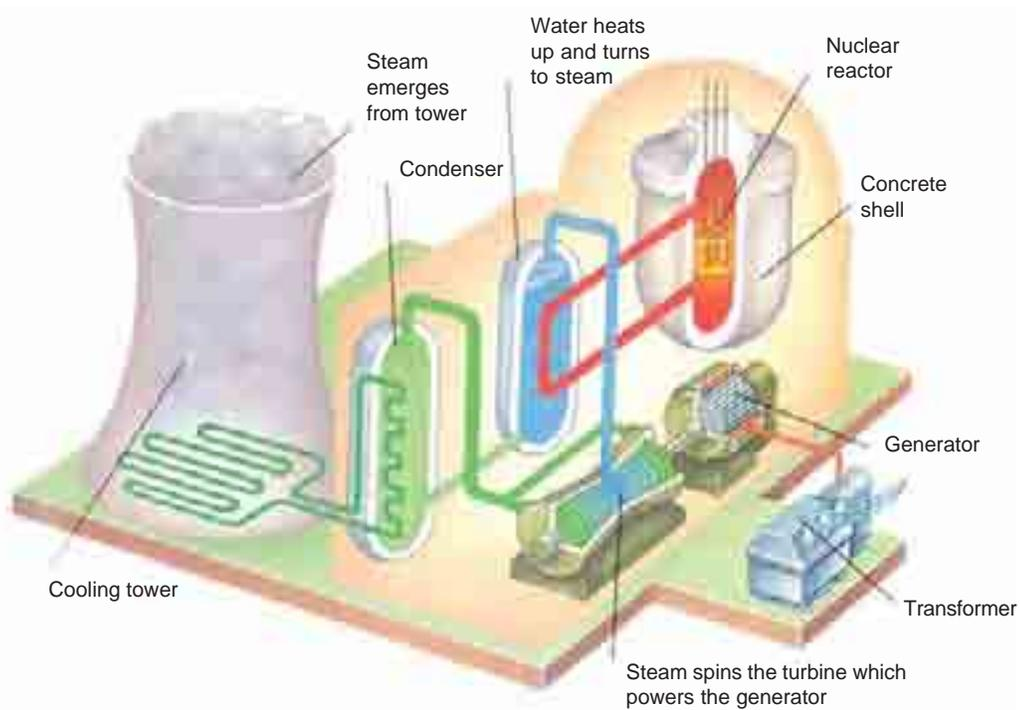
*In a nuclear power plant, steam is generated using the heat of nuclear reactions. Remaining function of steam turbines and generators is same as in thermal power plants.*
